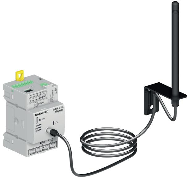
The remote antenna is connected to the DIRIS B-10L via a 3-meter SMA cable. The losses incurred by the antenna and the extension cable are about -4 dB.
