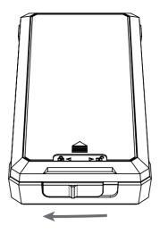
**Step 4:** Unscrew the battery door at bottom the of weather station.
