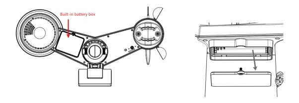
**Step 2:** Insert the 3 AA batteries according to the +/- polarity indicated. Then close the battery door.
