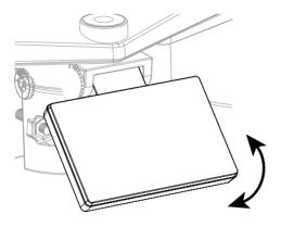
**Step 4:** Push the gear and tighten the screw until the gears are securely locked.
