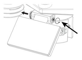
**Step 3:** Adjust the vertical angle of the solar panel (0°, 15°, 30°, 45°, 60°) according to the latitude of your location.
