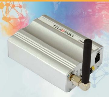
The RB800 terminal series is the complete modem solution for wireless m2m applications. Based on the high quality module, it is available as DUAL or QUAD band versions and offers high level GSM/GPRS/UMTS features in compact aluminum housing with all the standardized interfaces and optionally GPIO, SD memory card, backup battery or dual SIM option. Together with its small size and wide supply voltage range, makes it easy to integrate into all kinds of machines.
